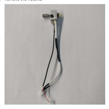
9. Remove the retaining screw on the hotend with a 2 mm hex wrench.
