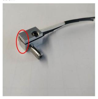
13. Reinstall the screw retaining the heating rod.
