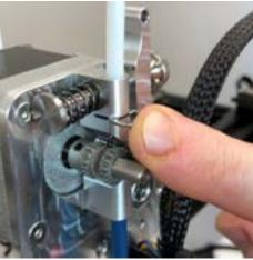
Insert the filament guide tube and secure it with the provided retaining clip
