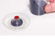
A durable plaster based resin is mixed with a pigment and cast in two stages to make dials with coloured caps
