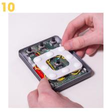
The silicone buttons are laid onto the switches
