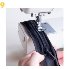
A zip is stitched into a loop with edges prepared so they join to case shells
