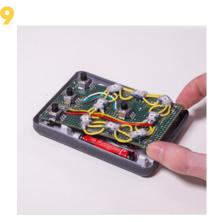
The circuit board and components are inserted
