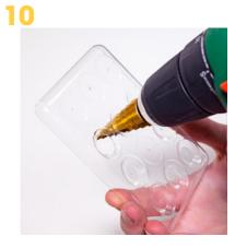
Holes for the various components are drilled out
