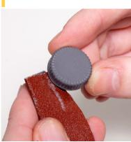
Any roughness or flash on the cast parts is sanded and polished
