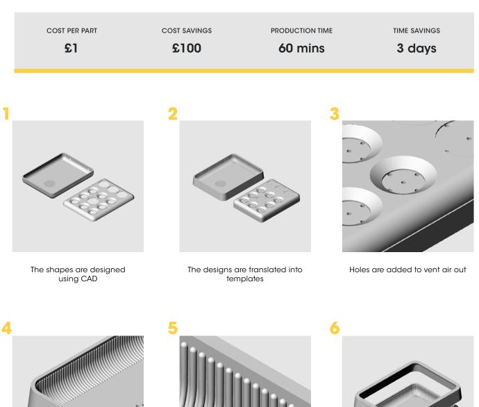
The texture on the bottom is designed so that there are no undercuts
