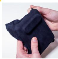
Napa leather is gently stretched around the PVC shells using a contact adhesive to bond the layers
