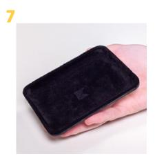
The tray is made with a black flocked HIPS sheet and trimmed using a scalpel and trim line
