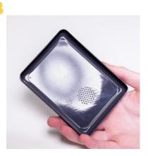
The shell's back is spray painted with frosting to diffuse the light from the LED behind
