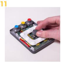
The dials are glued onto the potentiometers
