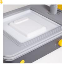
Both parts are formed from a PVC sheet and trimmed using a scalpel and a trim line
