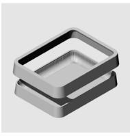
A two-part skirt is added to the lower template creating a lapjoint at the seam line between the upper and lower shells
