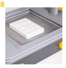
Both parts are formed from a 1.00mm transparent polycarbonate sheet
