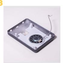
The part is glued into the base of the outer shell
