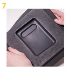
A sheet of EVA foam is formed around a slightly smaller template, this is done for both the front and back and trimmed at the seam line between the case shells
