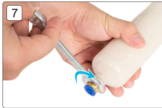
7 Tighten the pneumatic coupling with a wrench 使用扳手拧紧气动接头
