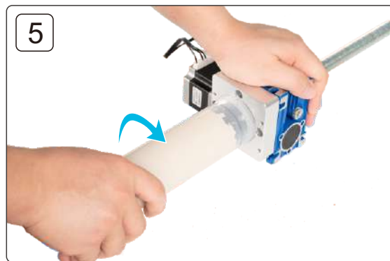
5 Tighten the barrel clockwise 顺时针拧紧料筒
