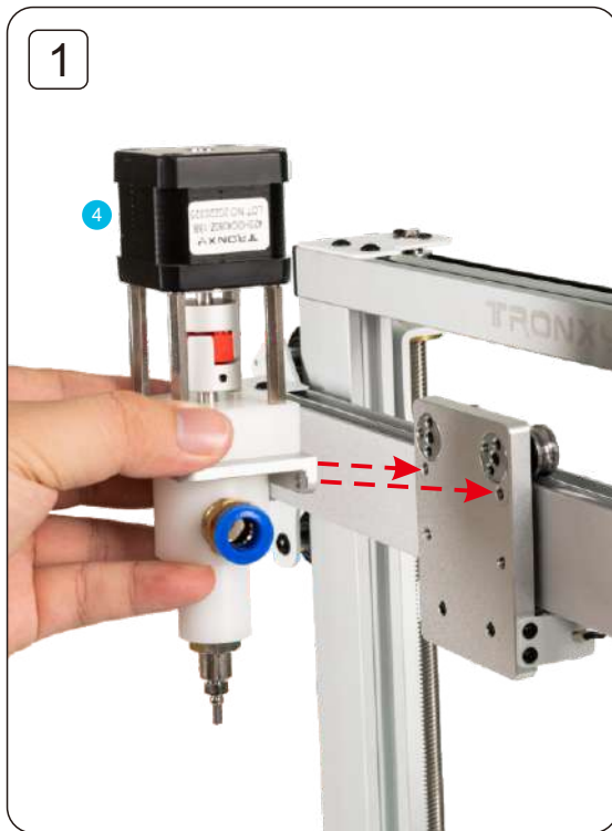
Install the print head on the slider as shown in the figure 如图所示, 将打印头安装到滑块上
