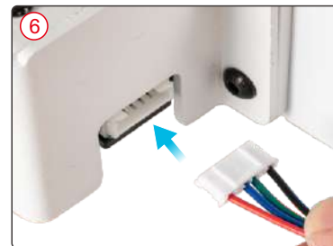
Plug in Z2 motor line 插入Z2电机线
