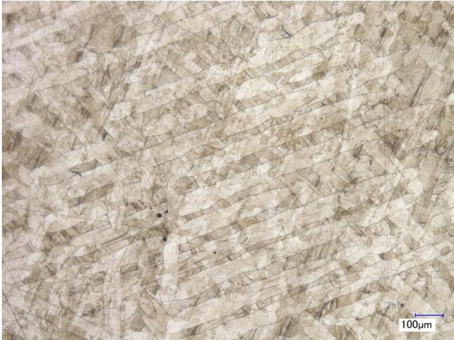
**Fig. 7** Etched plan view with visible melting traces and applied alternating exposure
