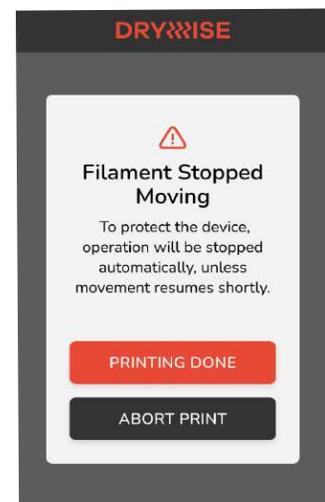
If for some reason the printer stops printing, the dryer will sense this and after giving the user time to fix the issue, it will abort the current operation if filament movement does not resume. Drying will also automatically stop once printing is finished.
