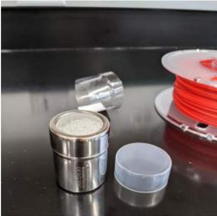
ⓘ Warning: twisting the plastic cap in the counter clockwise direction will remove the metal lid as well as the plastic cap. You risk spilling little desiccant spheres all over the place. Ask us how we know...
