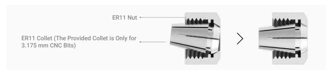
2. 2. Put on the CNC Safety Goggles. Insert the CNC Bit into the ER11 collet (Flat End Mill is required for our provided model). Keep pushing the CNC Bit until its end bottoms against the shell of the ER11 collet.
