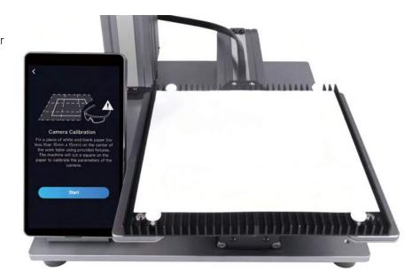
2. Tap **Start**, and the machine will use the engraved square to calibrate the camera.
