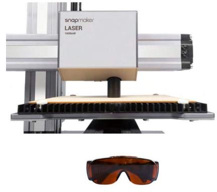
4. Tap **X-**, **X+**, **Y-**, or **Y+** to move the laser dot to where the Work Origin will be, and then tap **Set Work Origin** and **Run Boundary** to check if the work origin is proper. If not, reset the Work Origin and run boundary again.
