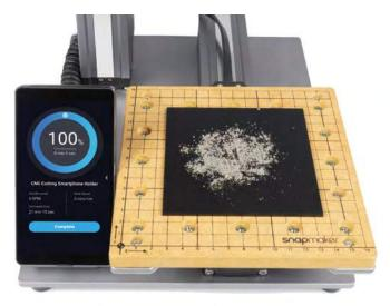
2. Clean the finished work and the machine with a dust collector, and then remove the finished work using the diagonal pliers.
