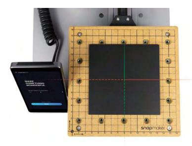
2. Attach the clamp set to the CNC Carving Platform, and then fasten the material by screwing the wing nuts.
