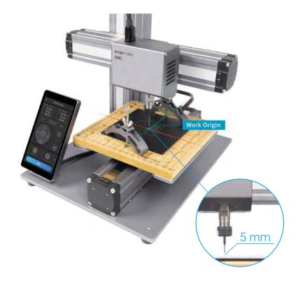
3. Place the Calibration Card or a piece of A4 paper between the CNC Bit and the material. Keep adjusting the height of the CNC Bit using **Z-** or **Z+** buttons until you feel slight resistance when you pull out the Calibration Card, and it should be wrinkled when you push it forward. Tap **Set Work Origin**.
