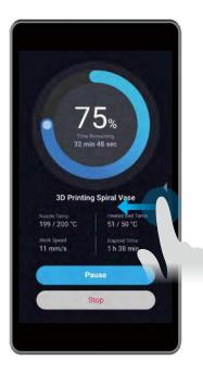
If poor adhesion occurs, swipe left on the printing progress screen and try adjusting the Z Offset. Or you can try leveling the Heated Bed again by selecting **Calibration**. Make sure the tip of the nozzle is clean before you calibrate the bed.
