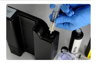
1.7 Cap all pigment bottles and syringes for reuse. Record remaining volume of each pigment on the designated location on the bottle label.
