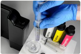
1.4 To use the syringes with different resins or pigments, pull the plunger from the body of the syringe and rinse with fresh isopropyl alcohol (IPA). Repeat if necessary.
