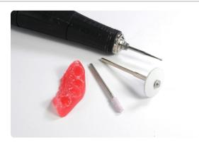
From right to left: gingiva mask on supports, supports cut, finished gingiva mask.
