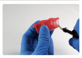
Small, sharp scissors can be used to cut the supports closer to the part as a second step.
