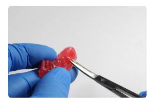
To remove supports on internal areas, we highly recommend using curved iris scissors.
