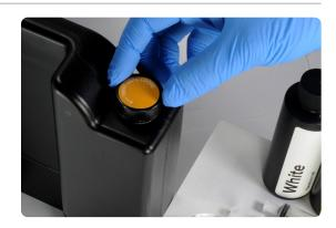
1.3 Remove 40 mL of the resin from the Flexible 80A cartridge using a glass cup or container and one of the provided 10 mL syringes.
