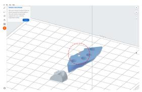
To easily rotate the part by 180 degrees, hover over the **Orient to Bounding Box** buttons within the **Orientation** tool. Select the button that will rotate the part so that the occlusal surface is facing toward the build platform.
