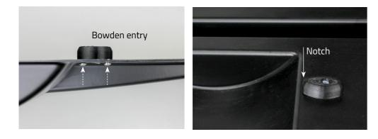
4.3 Insert the new teflon tube with the filament sensor into the "Bowden entry". Press until you feel that you have reached the end.
