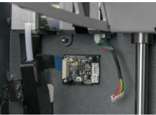
4.11 Connect the flat cable, and then connect the motor cable and the filament runout sensor cable as indicated the picture.
