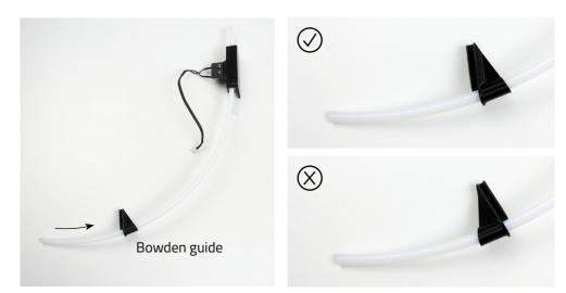
4.2 Screw the new printed part "Bowden entry" provided with the kit on the lateral covers with the two screws used in the step (2.9) as shown in the picture, with the orientation indicated (notch inwards).
