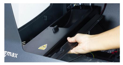
2.9 Unscrew the two screws at the bottom of the cover and remove the printed part "Bowden entry". Don't keep this part, as it won't be used again.
