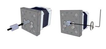
STEP 5: INSERT AND TIGHTEN 100k THERMISTOR.
