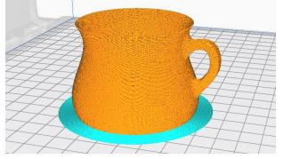
The brim width required will depend on the part geometry being printed. At least a 5-layer
