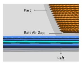
gap is 0.1mm (this value may vary slightly up or down based on your printer's make and model).
