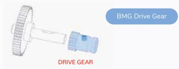
Make sure the set screw in the filament drive gear is seated against the notch in the shaft. Carefully tighten the set screw, the head is easy to strip.
