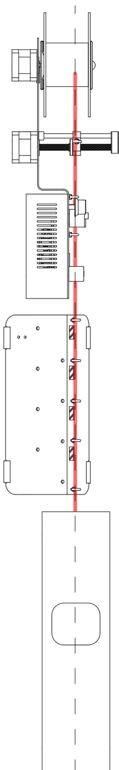
Place Felfil Evo, Fan Array and Felfil Spooler on a table and arrange them like in the pictures. All the machines must be aligned: align the Felfil Evo nozzle with the filament support placed on the Fan Array and Felfil Spooler.
