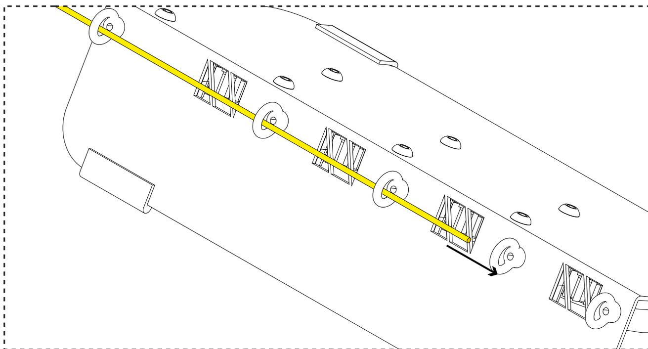
Insert the filament into the measuring system sliding up the little lever.
