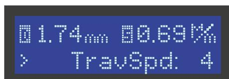
Travel distribution Speed. By default is set on "4". This parameter can affect the filament distribution.
