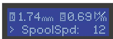
Spool Speed. Modify this parameter if the spool clutch is not working properly for your material, or if your extrusion flow is over 1,5m/m. Value in RPM.
