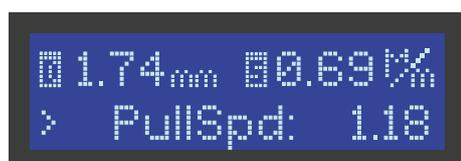
Puller wheels constant speed. Adjust this parameter according to your extrusion flow.
