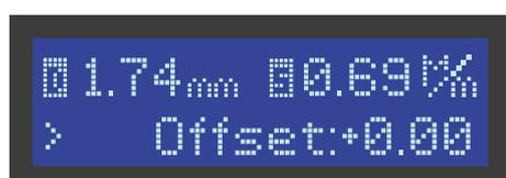
It allows to calibrate the measure, use it if the real measure is different from the one you read. Example: measure an hex key using a caliper. Then insert the hex key into the measure system, if the measure is not the same, regulate the offset.
