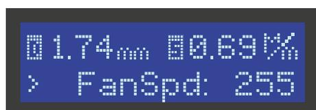
Fan Speed. You can modify the airflow of fan array if necessary.
