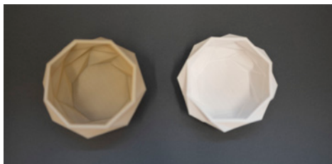
Examples of printed part shrinkage after drying.
