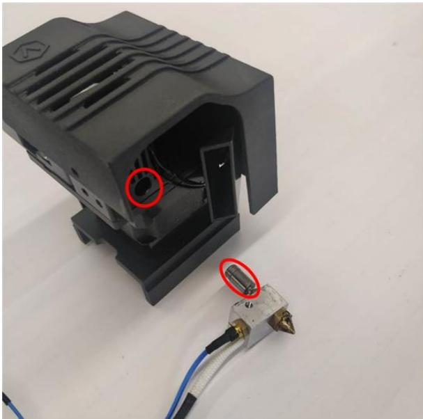
15. Once the hotend is inserted fully into the extruder, use a 2 mm hex wrench to tighten the screw to retaining the hotend.
