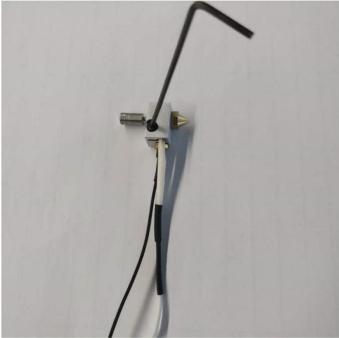
10. Once the retaining screw is loosened, the heating rod should be able to slide out.
