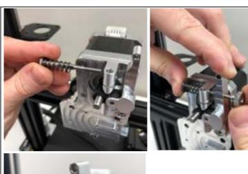
Screw in the lever adjusting knob until the pin is flush with the knob.
