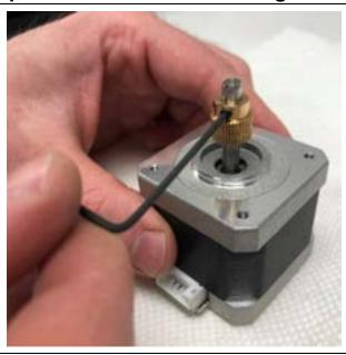
Remove the extruder gear using the 1.5mm Allen wrench
