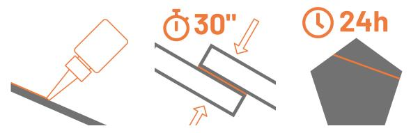
The contact surfaces should be dry and free of contamination like oil or grease. Apply the adhesive sparingly to one surface. Press together immediately. Hold in place for 15 to 30seconds until bond sets. Let product rest for a while to give the glue time to fully harden. After 24h the bond has been fully set.
