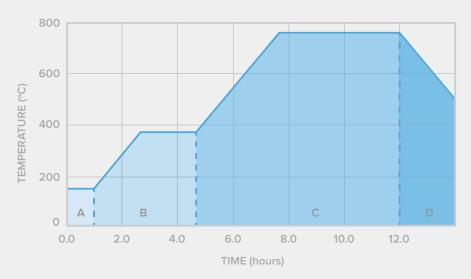
The Standard Burnout Schedule is designed to provide the maximum possible investment strength and complete burnout of the finest details using R&R Plasticast or similar investment materials. Use this schedule as a starting point and make adjustments as needed.
