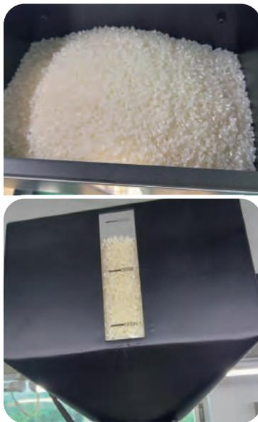
2 The pellet (diameter 1.0~5.0mm) material is loaded into the feeding barrel.
