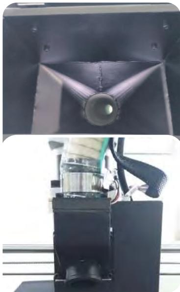
1 Check whether the feeding tube is connected properly.
