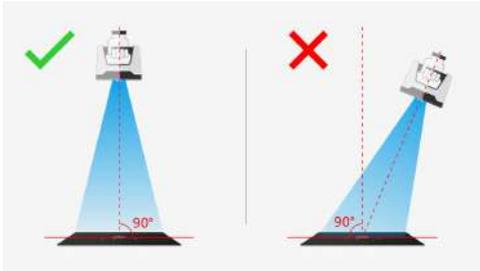
2. After picking up the scanner, move it above the calibration board. The scanner should be positioned vertically, facing directly towards the table, in the same direction as shown in the diagram. Ensure that the crosshair projected by the scanner is positioned within the white square at the center of the calibration board.
