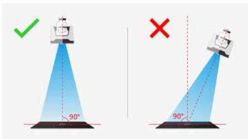
2. After picking up the scanner, move it above the calibration board. The scanner should be positioned vertically, facing directly towards the table, in the same direction as shown in the diagram. Ensure that the crosshair projected by the scanner is positioned within the white square at the center of the calibration board.
