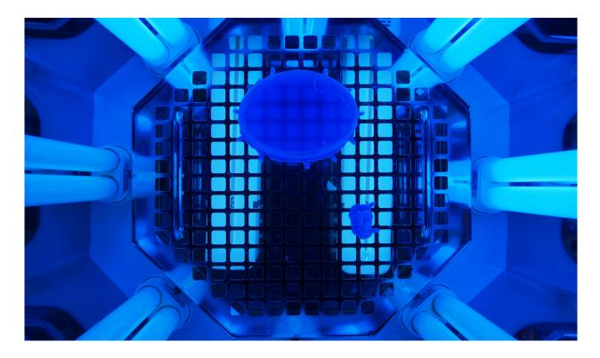
Post-cure the parts under 405 nm light and heat until the surface is hard and rigid. Rotating parts ensures an even post-cure. Form Cure will automatically rotate parts, but if using another method, it may be necessary to manually flip or rotate parts during the post-cure.
