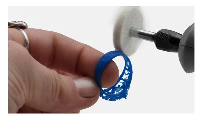
Polish the surface using polishing paper or a rotary tool with a buffing attachment. Do not finish the print with mineral oil after sanding.
