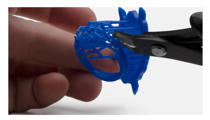
If necessary, carefully remove support material from your print. Using fine sandpaper (400 grit and above), gently sand away support marks.
