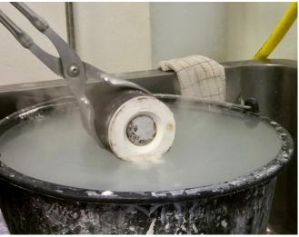
Remove the mold from the furnace and cast metal. Centrifugal or vacuum casting processes can be helpful in quickly filling the mold.
