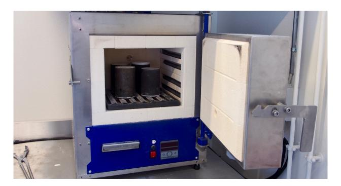
Place the casting flask in a cold furnace and heat using the burnout schedule as a guide. Make adjustments depending on the investment instructions, flask size, and material. If starting the burnout with a hot oven, make sure that the flasks have been resting for at least 5 hours, otherwise the plaster might crack when the water expands and turns into steam.
