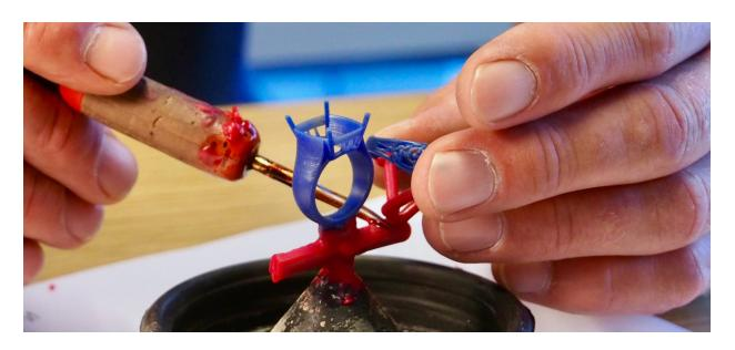
Add wax sprues and gates to the print, similar to lost-wax casting. Ideal positioning varies with part geometry.
