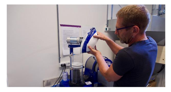
Weigh and mix the investment, and pour it into the casting flask according to the manufacturer's instructions. For example, instructions for R&R's Plasticast with BANDUST.
