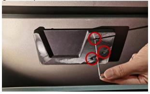
3. Set aside another 3 screws to affix the new right shaft sleeve holder. The mounting procedure is identical to the 2.5 kg left shaft sleeve holder; align and fasten the 3 screws on the 2.5 kg right shaft sleeve holder. The installation of the two shaft sleeve holders is complete.
