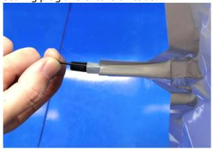
4. Finally, enshroud the sealing plug with a sealing cover, and ensure that a short length of extension tube is captured within the sealing cover. The sealing of the filament bag is complete.
