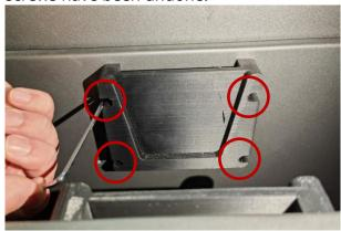
2. Carefully bring the new 2.5 kg left shaft sleeve holder into the position of the original holder, and align the 3 screw holes of the holder with those of the cartridge inside the machine. From the 8 screws removed in the previous step, set aside 3 to use now. Use a 3 mm hex wrench to fasten the 3 screws, starting from top to bottom.
