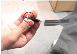
3. Gently pull the end of the filament outwards to ensure that it may not recede into the sealing plug and extension tube.
