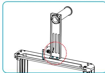
② Secure the material rack and filament detection assembly onto the gantry frame, align the screw holes and lock it with M5\*8 screws;
