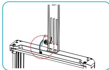
③ Connect the filament detection switch.
