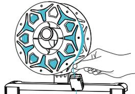
③ Thread the straightened filaments through the filament detection switch;
