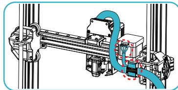
② Following the wire label instructions, first insert the extruder line into the cable fixing clip, and then connect the X-axis motor;
