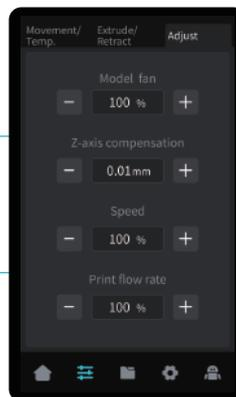
Use the preparation interface to set functions such as axis movement, temperature control for filament extrude/retract, and model fan.
