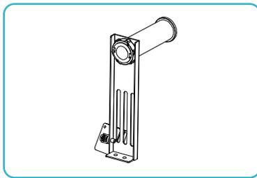
① Install the material rack and material barrel according to the diagram;
