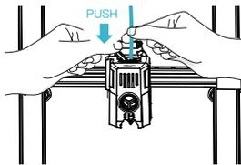
④ Gently press the extrusion clamp and push the filaments that have passed through the filament detection switch through the hole to the bottom of the heat break, until there is some excess filaments protruding at the nozzle.
