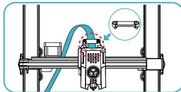
① First insert the nozzle wire into the nozzle adapter plate , then install the FFC fixing clip assembly, and use M3\*8 screws to fix and lock it;
