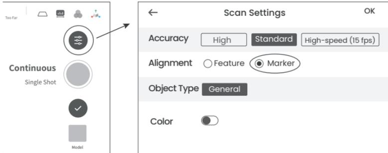
1. Place the Markers (or Magic Mat under the object) on or around the objects' surface irregularly and ensure there are at least 5 Markers per frame for the entire scan, or the scanner will lose track.
