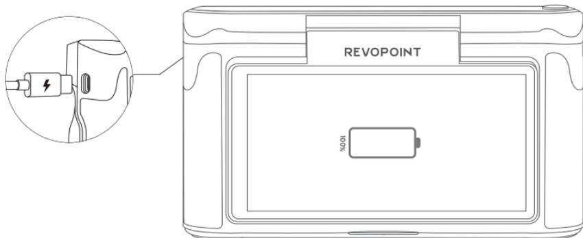
**Step 2:** Long-press the **Power Button** (5s) to turn on.
