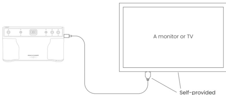
**Method 2:** Use the DP to HDMI Adapter (included with MIRACO Pro) to connect MIRACO to an HDMI cable on a TV or monitor.
