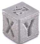
The minimum final dimensions are a cube of 7mm. A smaller piece could have non protruding edges.
