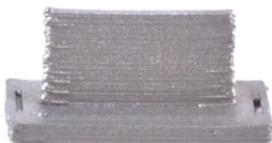
The width of the wall must be proportional to the width of a layer, since such a thin wall does not have an infill.
