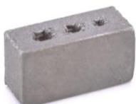
The minimum size of a horizontal hole is 1,5mm in diameter. A smaller hole may be closing up.
