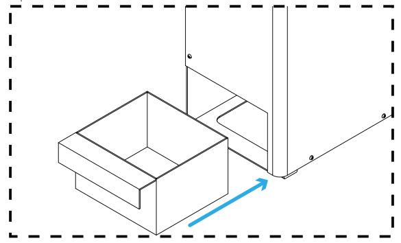
In order to use the Shredder, the binder must be in position since a safety sensor prevent the starting when its open
