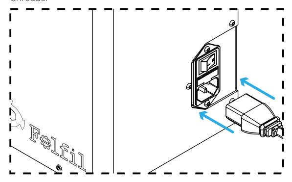
Turn on the Shredder, pushing the power switch just above the power plug
