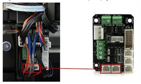
Insert the cables of the Heating Rod into the terminal and tighten the screws to fix.
