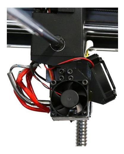
Grab the connector of the new Fan by tweezers out from the top to help it go through the Mounting Block.
