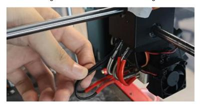
4. Install the new Fan Replace a new Fan.
