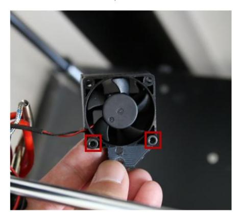
Preparation for WiringUnplug the cable of Side Cooling Fan from extruder board.
