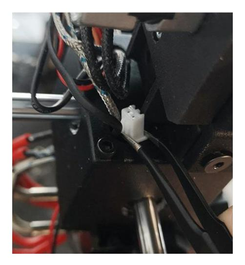
Plug the side fan cable onto the terminal where you unplug the old cable.
