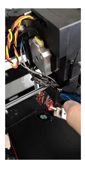
Loosen the screws marked in following image. And remove the Heating Rod cables from extruder board.
