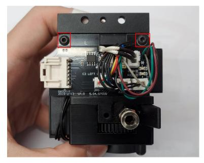
22. Put the front cover back to the extruder, and use the 2mm hex wrench to screw the two screws back.
