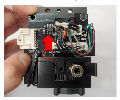
11. Unplug the two cables from the slots marked in red as shown in the picture below. *Note:* Unplug the cables from the first and the third slot of all three slots.
