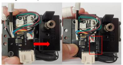
21. Plug the two pins into the controller board.
