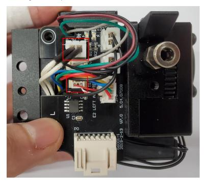
22. Using a 2mm hex wrench to tighten the two screws and securing the extruder connection board to the extruder.
