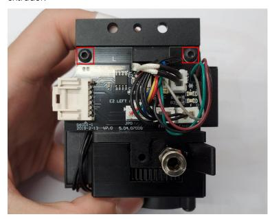
10. Gently pull out the extruder connection board in the direction of the arrow shown below. Be mindful of the small protrusion holding it in place.
