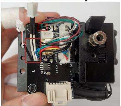
20. Plug the small protrusion of the board into the hole on the extruder.
