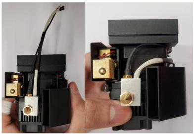
19. Place these cables into the cable management slots of the extruder controller board.
