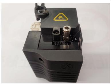
7. Using a 2mm hex wrench to loosen and remove the two screws securing the extruder connection board cover to the extruder.
