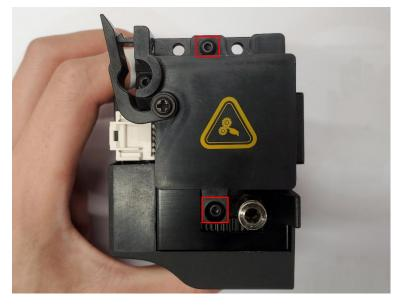
8. Using a 2mm hex wrench to remove the two screws securing the front cover to the extruder, and remove the front cover.
