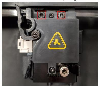
25. Insert the extruder connection cable back into the extruder, and press the fixed buckle to hold the cable in place.
