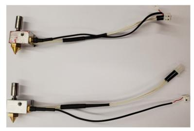
16. Plug the new hot end assembly into the extruder.
