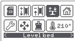
The printer will take a reading from the centre of the bed and will move to the first front left point. If the red LED of the sensor does not light up or flash, it means that the distance between the bed and the extruder is incorrect. To correct it, you will need to turn the knurled wheel below that corresponds to this point, so that the bed moves on the Z axis until the LED stops blinking. This point will be levelled when the red light remains on.
