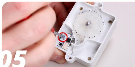
**05** Remove the screw holding the flow control board using a 2mm hex driver.
