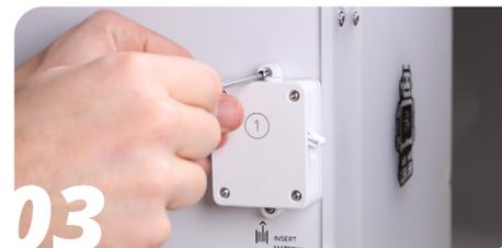
**03** Remove the top and bottom screw using a 2mm hex driver.
