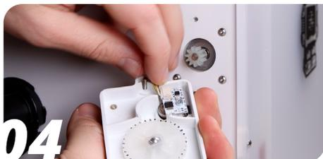
**04** Disconnect the flow control wire, if present on your printer.
