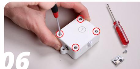
**06** Unscrew the four screws holding the extruder together using a 2mm hex driver.
