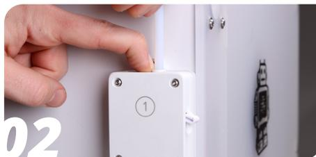
**02** Push down on the collet and pull the bowden tube out.
