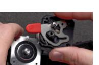
Remove the extruder assembly from the motor.
