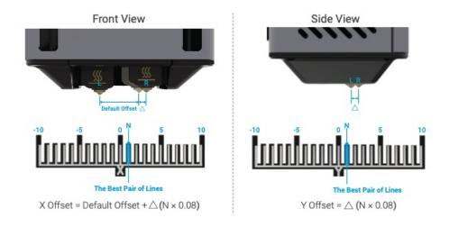
However, some printers remove the "Default Offset" or the "Nozzle Distance" from the offset before being entered into the printer settings. In these cases, the X Offset follows the formula below. For these printers, we need to know the "Default Offset" or the "Nozzle Distance" ahead of time so the CXC software can calculate the correct number to enter into the printer settings.
