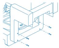
4 Using the 5 mm hex wrench, install 4x gantry screws with washers
