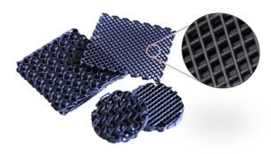
Scaffolds printed with Filament-Eco 25Carbon
