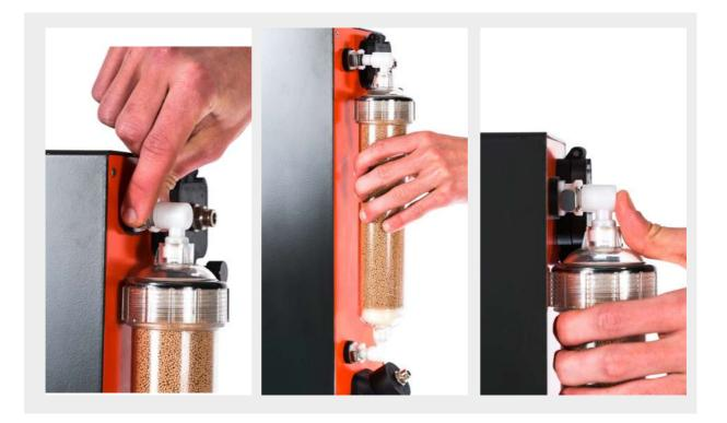
You are done with the desiccant cartridge replacement and can proceed with normal drying operation.
