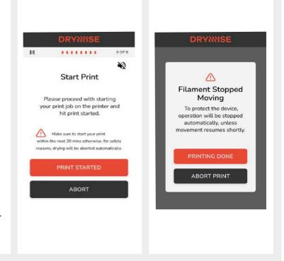
If for some reason the printer stops printing, the dryer will sense this and after giving the user time to fix the issue, it will abort the current operation if filament movement does not resume. Drying will also automatically stop once printing is finished.
