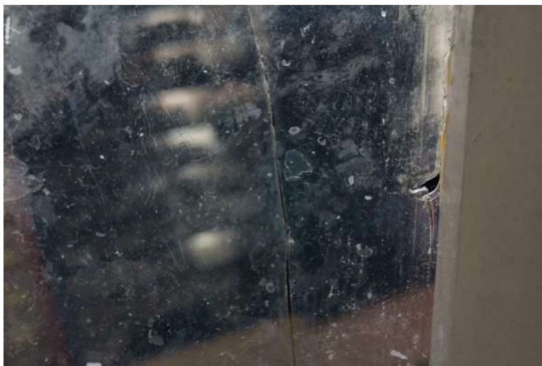
An extreme case of FEP film damage
