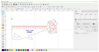
3. Set different color blocks for different processing techniques to distinguish the graphics. Click to select the corresponding graphics, move the mouse to the color block bar and select the corresponding setting and color.
