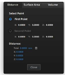
Calculate the distance between two points or markers on the surface of the scanned model.
