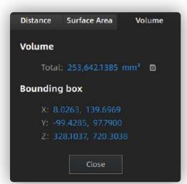
Calculate the volume of Meshed data with a unit of mm<sup>3</sup>. When you switch to Volume, the volume of the scanned model and the coordinates of corresponding bounding box will show themselves.
