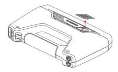
2. Insert the Color Pack and lock it with a rotary lever.
