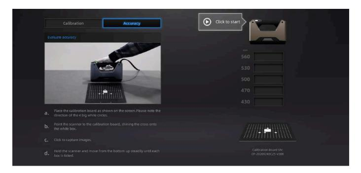
1.Place the calibration board with the front side (black background with white dots) facing up, flat on the table, and align it in the same orientation as shown in the diagram.
