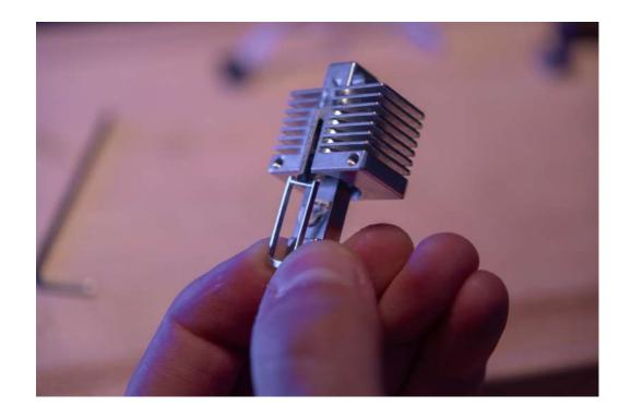
**Step 3:** Insert your heater into the heater adapter
