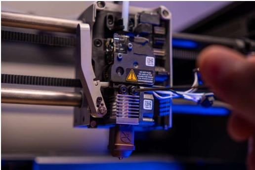
**Step 3:** Route all the loose cables through the plastic wire clip
