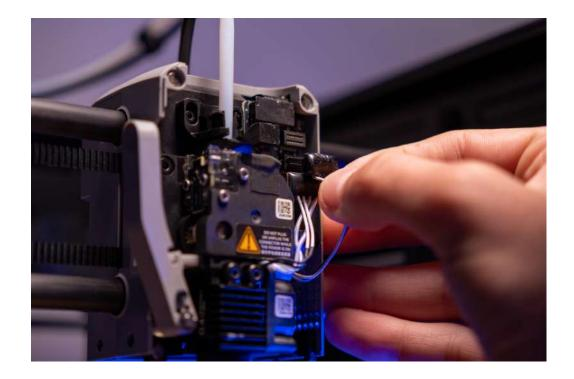
**Step 3:** Use the 2mm hex key to unscrew the 2 screws that are near the top of the hotend's heatsink
