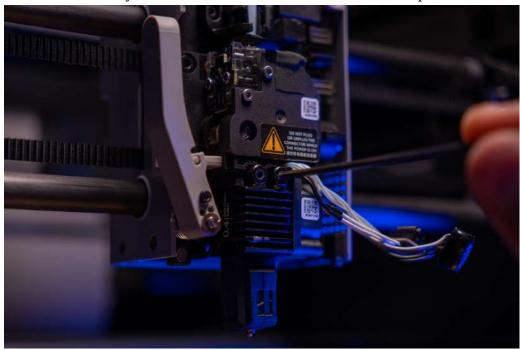
**Step 4:** Carefully and gently move the wires out of the plastic wire clip and remove the complete hotend assembly.
