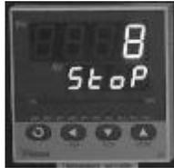
② The set points of the step StEPXX are displayed (C XX temperature in °C, and t XX time in min).
