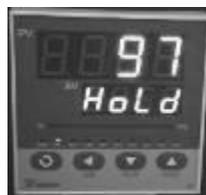
In Hold state, press the
