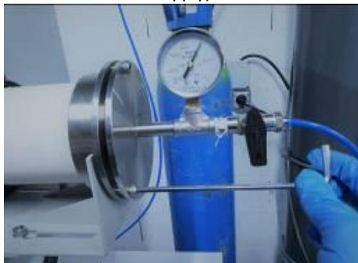
Left: Outlet flange (OD 10mm connection to the vacuum pump or to the bubbler)
