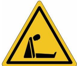
Inert gaz such as Argon are dangerous due to the asphyxiation hazard. The working area must be ventilated with an adequate venting system. Using of an oxygen gaz monitor is
