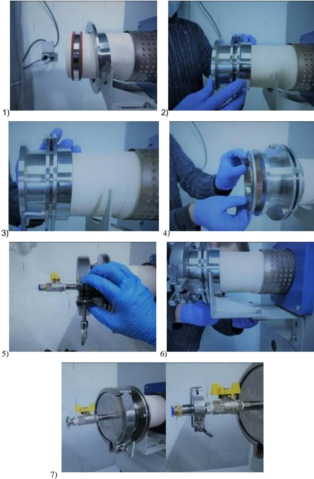
Adjust the position of the tube holders under the flanges, they must be in contact with the flanges.
