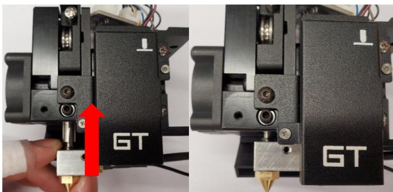
17. Tighten the socket screw.
