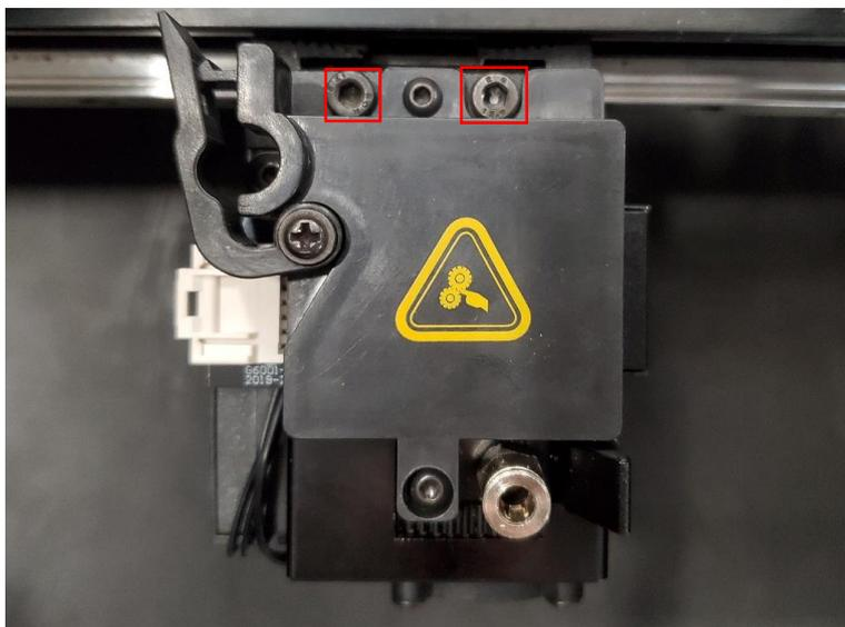
6. Remove the extruder from X-axis, and move it to a working desk.
