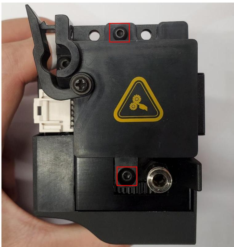
24. Put the extruder back to the X-axis, and tighten the two screws that holds it on the X-axis.
