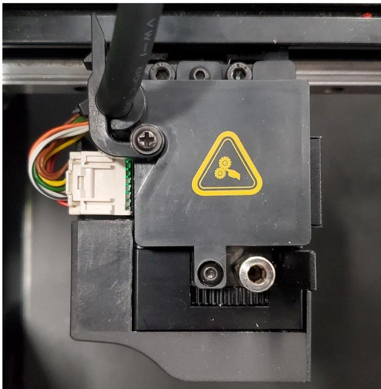
26. Turn on the printer and run the five-step wizard to calibrate, it is recommended to adjust the height of the left and right nozzles as well. (For more information please refer to the tutorial: [Manual E2 - How to Adjust the Height of Left and Right Nozzle – V1.0](#)).
