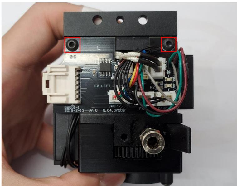
10. Gently pull out the extruder connection board in the direction of the arrow shown below. Be mindful of the small protrusion holding it in place.
