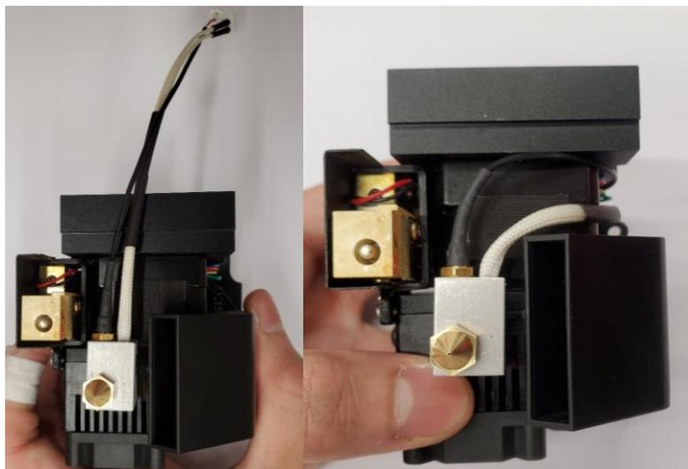
19. Place these cables into the cable management slots of the extruder controller board.
