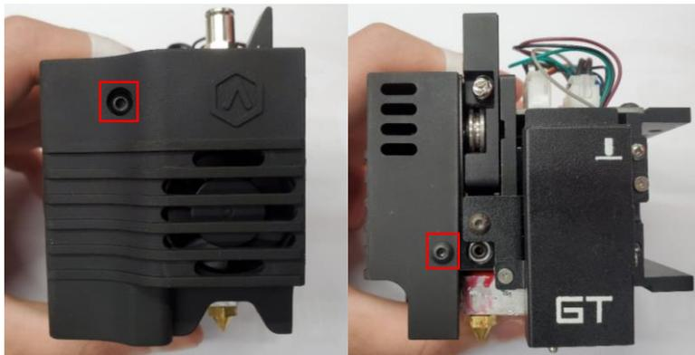
9. Using a 2mm hex wrench to remove the two screws securing the extruder connection board to the extruder.
