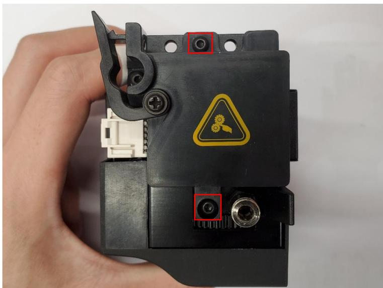
8. Using a 2mm hex wrench to remove the two screws securing the front cover to the extruder, and remove the front cover.
