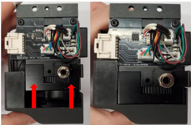
23. Put the extruder connection board cover back to the extruder, and use the 2mm hex wrench to screw the two screws back.
