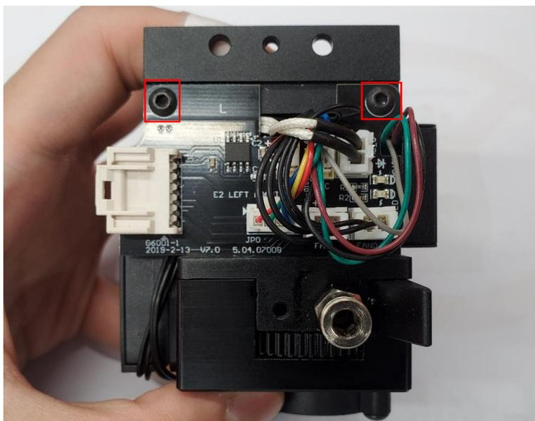
22. Put the front cover back to the extruder, and use the 2mm hex wrench to screw the two screws back.
