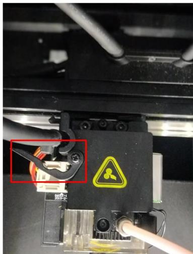
4. Unplug the extruder connection cable from the board by pressing the small plastic connector down, and gently pulling the connector out.
