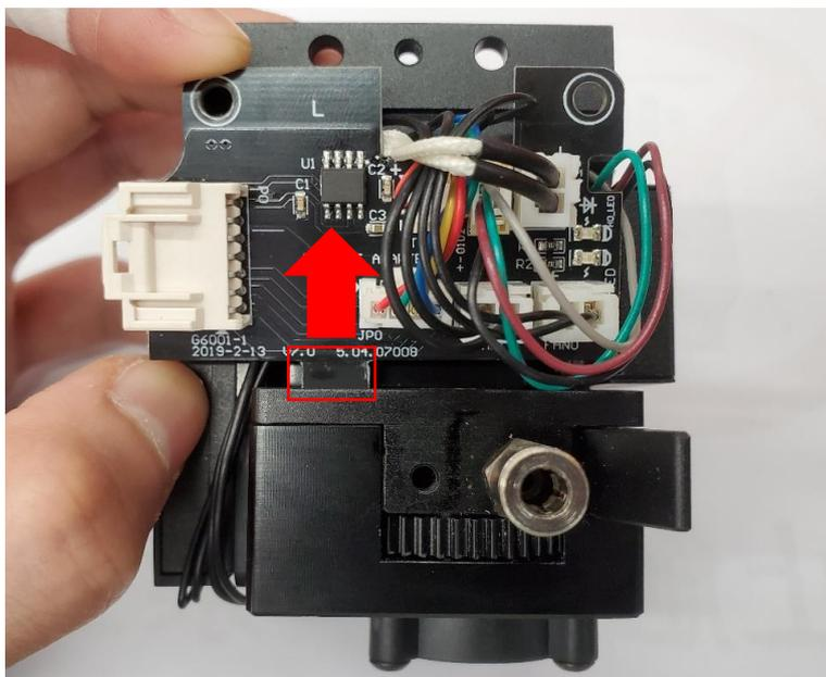
11. Unplug the two cables from the slots marked in red as shown in the picture below.
