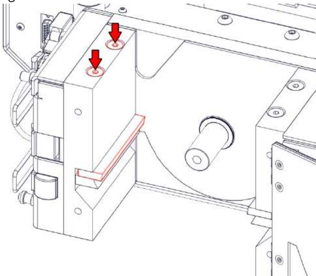
The left stationary knife can now be used as a reference for adjusting the rotary knives
