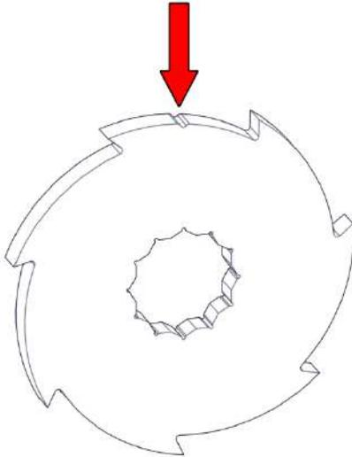
Step 6) The recommended configuration for 7 teeth blades is to stack each subsequent blade one-sixth turn with respect to the previous blade of the same shaft. In case of a 3-teeth-blade: use steps of 30 degrees ( $1/12^{\text{th}}$  of a turn). These sequential turns can be done either clockwise or counterclockwise as long as it is done consistently for both shafts.
