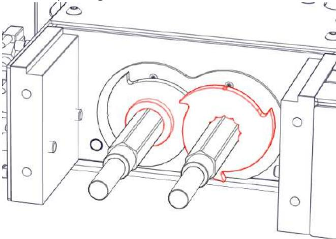
Step 4) Slide a shredder spacer on the left shaft opposing the shredder blade.
