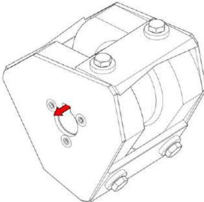
Step 8) Locate the key inside of the shaft
