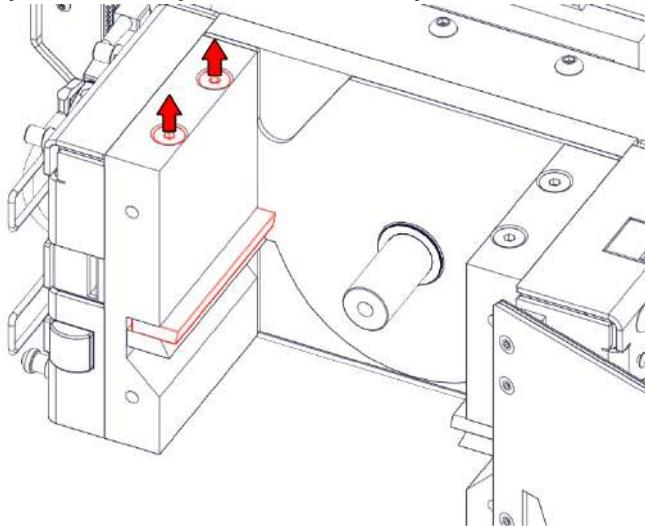
Step 3) Adjust the position of the left Stationary knife by tightening or untightening the set screws from the side using a 3mm Allen key. A good starting point is to offset the cutting edge of the stationary knife by 10mm with respect to the block it is mounted on. Use the two set screws to carefully manipulate the left stationary knife.
