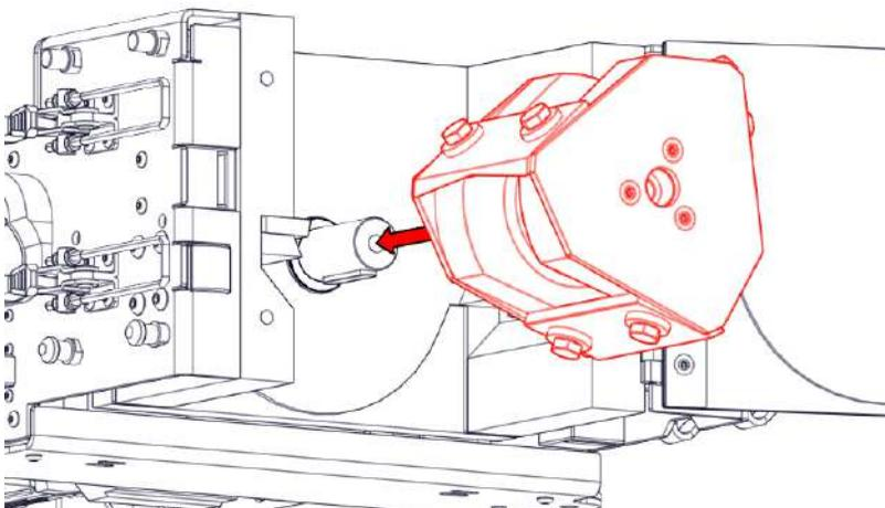
Step 8) Manually turn the rotor so that the cutting edge of one rotary knife is touching the cutting edge of the left stationary knife. Use a thin piece of paper or set the right gap between the rotary knives and the left stationary
