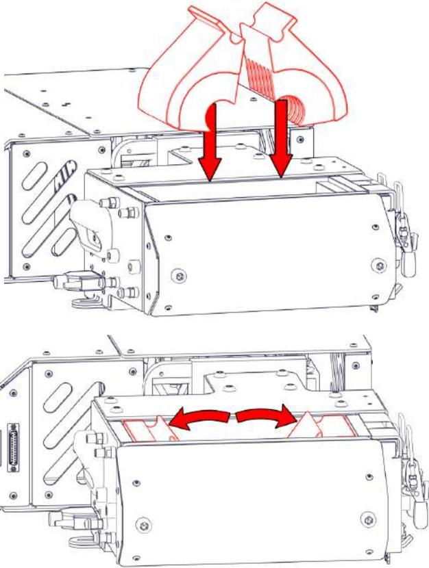
Step 2) Tighten the bolts on the side using an 8mm Allen key. This will keep the scraper combs in place. Don't tighten it too.
