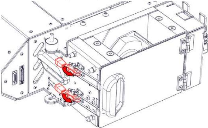
Now, open the toggle clamps and the granulator door will be pushed open by a spring loaded element. The door is pushed open to ensure that the safety sensor will be disengaged.
