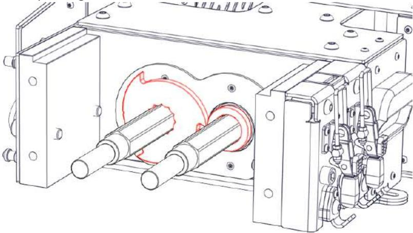
Step 2) Slide one shredder spacer on the right shaft opposing the shredder blade
