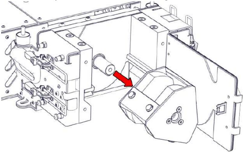
Step 6) When installing the rotor, it is important to properly clean the cutting chamber first to ensure proper alignment of the rotor.
