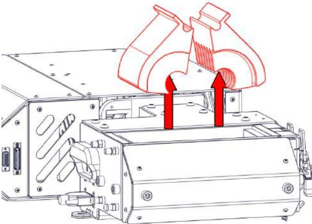
For installing the Scraper combs, the same steps can be done in reverse as shown above.
