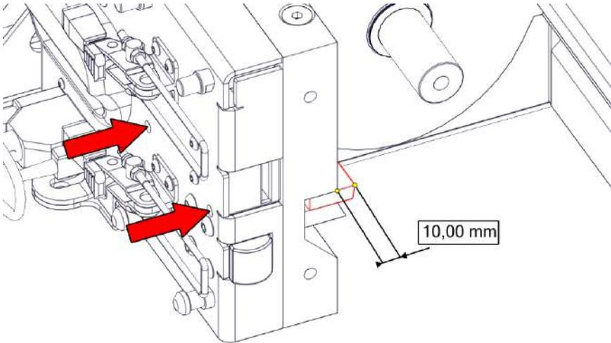
Step 4) Fix the left stationary knife in position by tightening the two bolts on top of the machine. Make sure the stationary knife does not move while tightening.
