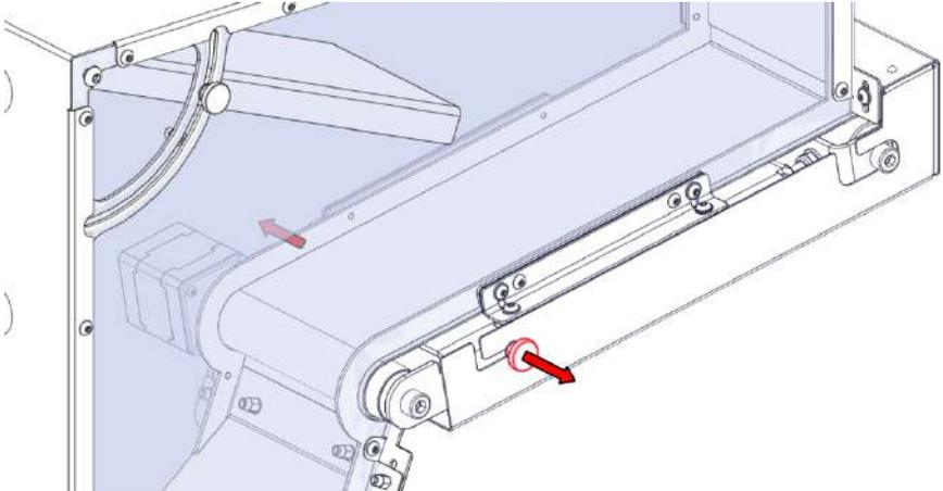
Step 2) Remove the cover by first sliding the cover horizontally followed by a vertical movement down.
