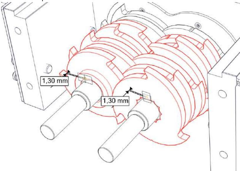
Step 9) Slide the front plate back on the shafts. Make sure the front plate is cleaned properly around the cylindrical bushings.
