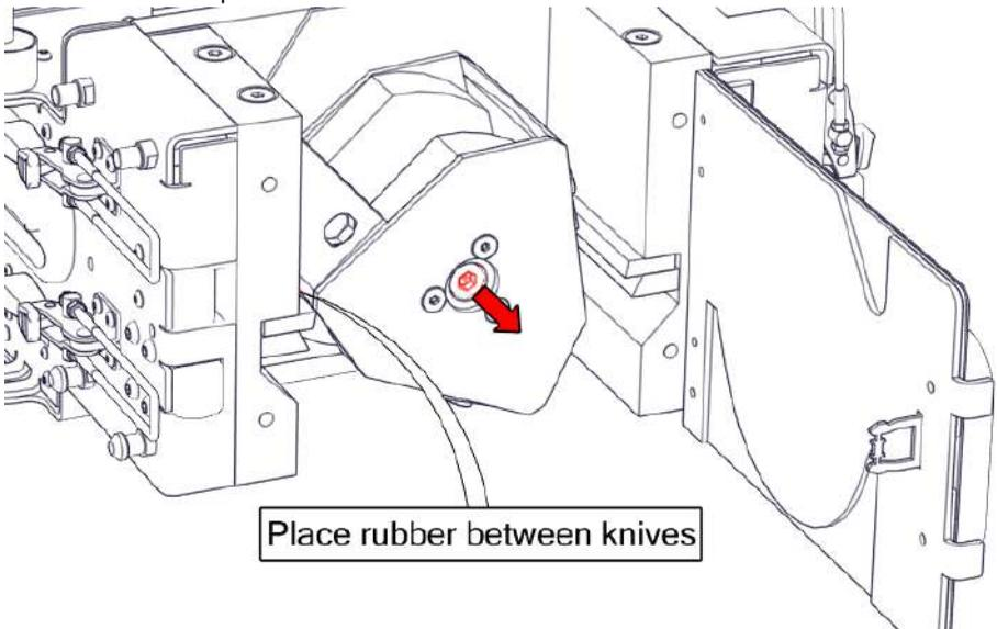
Step 5) Carefully slide the rotor out of the cutting chamber.
