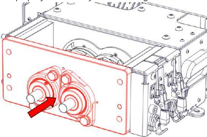
Step 10) Start by placing one thin nut per shaft and tighten the nuts a little bit at a time. Even tightening is important to avoid imbalances in the stacked blades.
