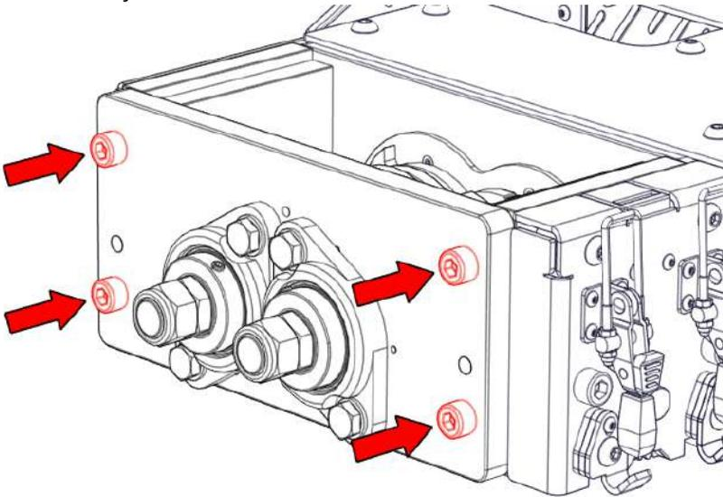
Step 13) Mount the black casing plate back on the machine by screwing in the two bolts also using a 8mm Allen key.
