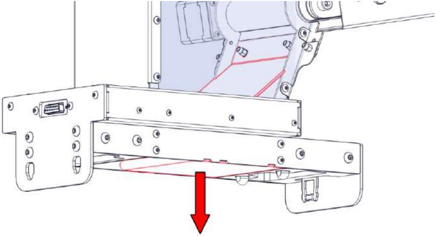
When reinstalling, keep in mind to insert the tabs inside the cut-outs before tightening the screws.
