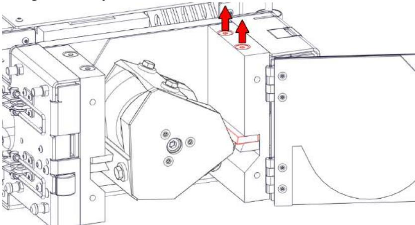
Step 15) Use a 3mm Allen key on the right side of the machine to adjust the right stationary knife with respect to the rotary knives. Use a thin piece of paper to set the right gap.
