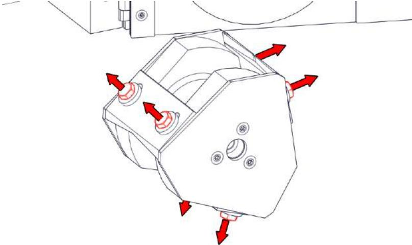
Step 7) Place the rotor with the free moving rotary knives back in the machine and lock it on the shaft.
