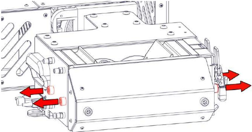
Step 3) Carefully pull the scraper comb up and lift it out.
