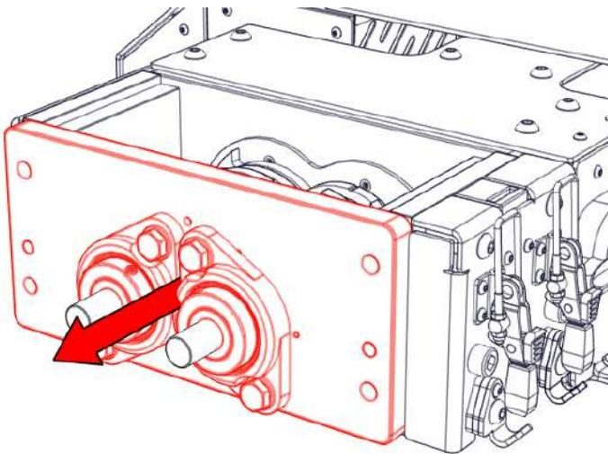
Step 5) Now, you can remove the shredder blades and spacers one by one.
