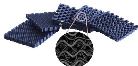
Scaffolds printed with Filament-Eco Graphene
