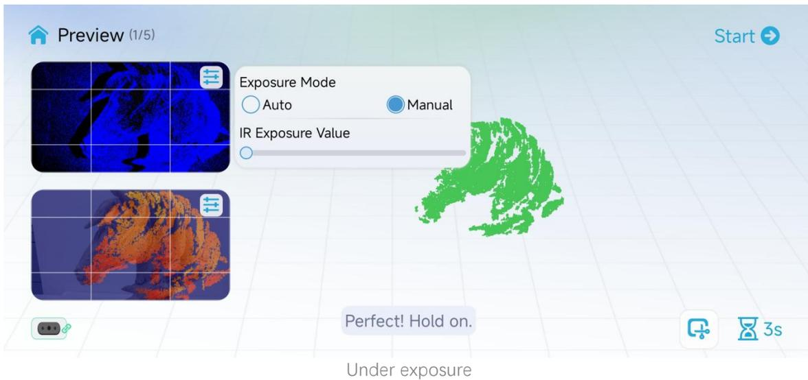
The RGB/depth preview window supports adjusting the RGB exposure mode (auto/manual, default auto). If you find that RGB is overexposed or too dark, you can appropriately adjust the exposure level. This preview window also supports the display of depth images, which can be superimposed on RGB images by adjusting the depth translucency.
