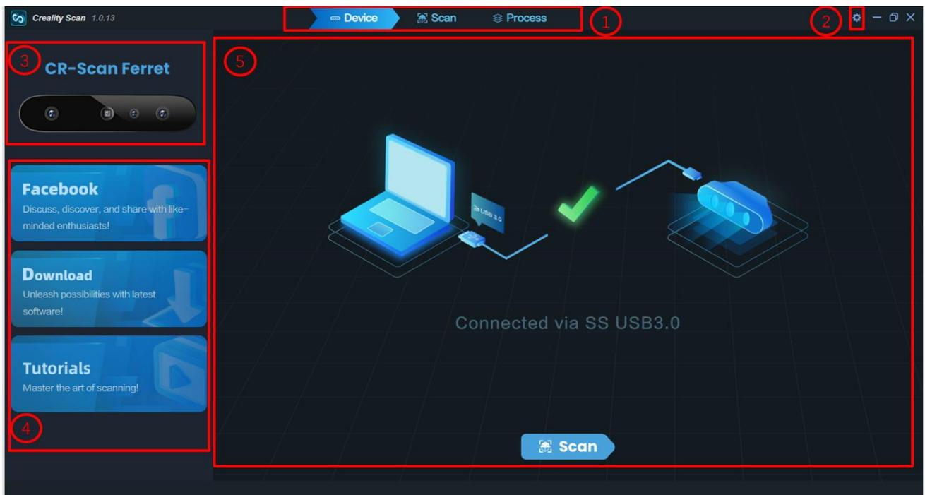
After opening Creality Scan, confirm the device connection status.
