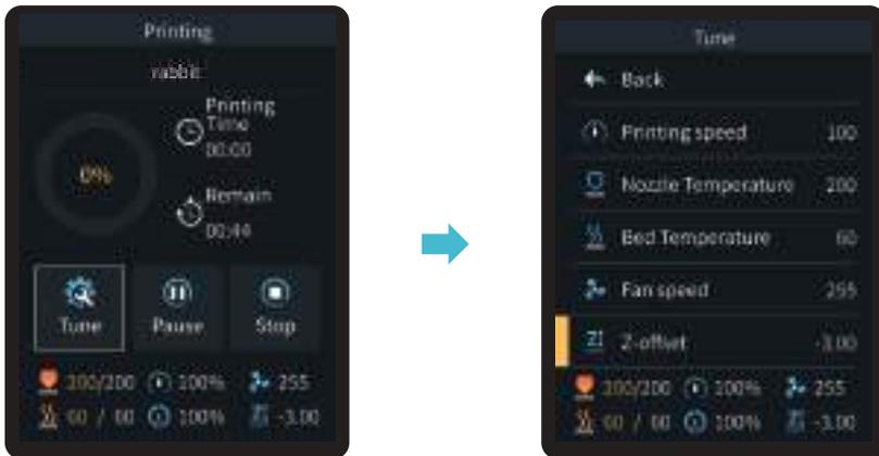
For levelling effect, please refer to the operation and try to maintain a distance of approximately 0.1 mm between the printing platform and the nozzle.
