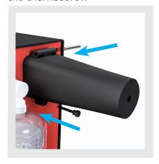
b) Remove the thumbscrew and the dowel pin
