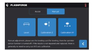
Manual leveling mode: Execute platform leveling, Z-axis calibration and X, Y axis calibration in turn. This is a complete set of leveling and calibration operation procedures.
