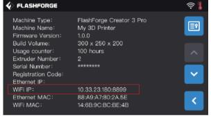
2. Click [Tools]-[Setting]-[About] in turn in the main interface to query and record the equipment Wi-Fi IP address: 10.33.23.180 (The example is for reference only. The local IP address shall prevail.)
