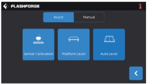
9-point leveling function: when the printing flatness is still poor after the platform leveling and XY/Z axis calibration, this function can be used to compensate for better flatness;
