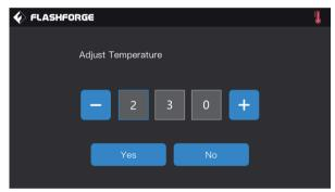
8. Filament feeding operation: Click the [Tools]-[Filament] button on the screen in turn, and set a reasonable heating temperature according to the required temperature value of the material; Operate according to the screen prompts, and wait for the nozzle to extrude uniform filament smoothly.
