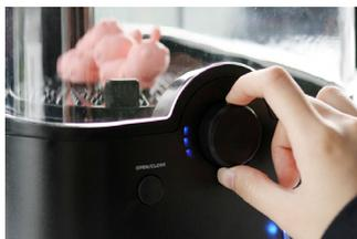
You can turn the chamber lighting on and off by pressing the Chamber Light button. The color of the mist lighting can also be adjusted by pressing the control knob and then rotating it until you see the desired color.
