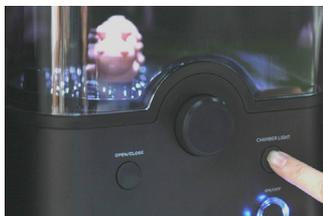
You can let the Polysher™ run automatically until the timer expires, or you can stop polishing at any time by rotating the control knob counterclockwise until no time indicators are shown. In either case, tones will sound to let you know the smoothing cycle has finished. The Polysher™ will then begin its "clearing cycle" during which the chamber fan is run at high speed to clear the mist from the chamber.
