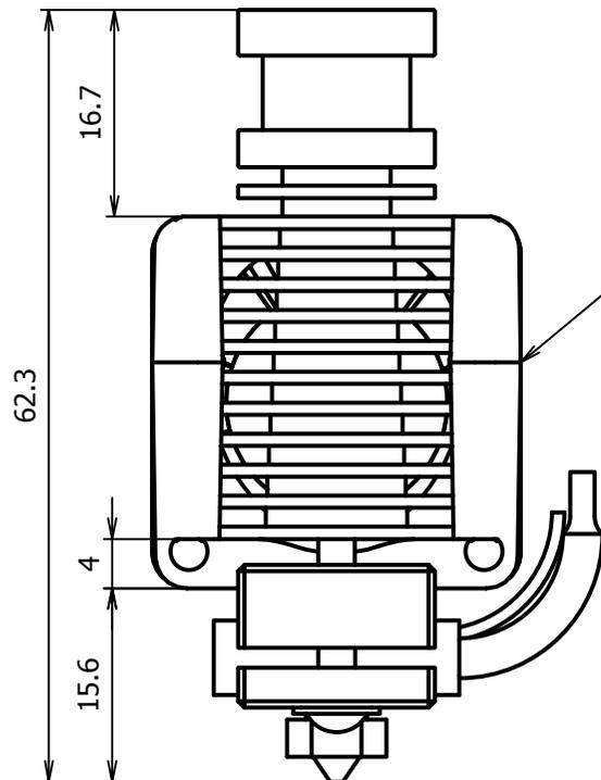
NOTE: THE DUCT CAN BE MOUNTED EITHER WAY UP
